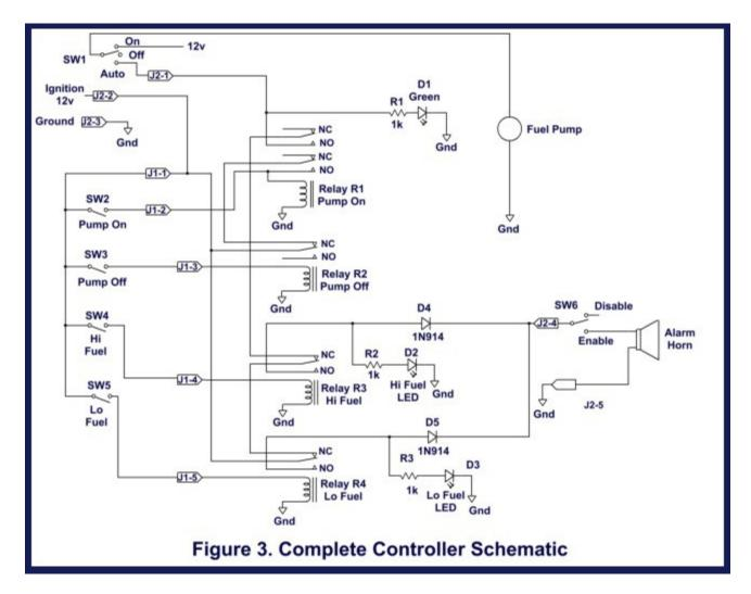
Note that there are two minor shortcoming to the controller design that could be corrected at the cost of added complexity. First, if the pump switch is in the "ON" position and the engine ignition is off, there will be no alarm if the tank overflows. Second, if the alarm is sounding, I have to look in the engine room to determine the cause. It would be nice to add external LEDs for the Day Tank status.
